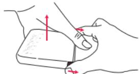
While holding the 2 latches in the down position, place your free hand under the refill and your thumb on the trigger (as shown on the diagram). Using your thumb, pull the refill up towards you to remove it.
