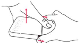
While holding the 2 latches in the down position, place your free hand under the refill and your thumb on the trigger (as shown on the diagram). Using your thumb, pull the refill up towards you to remove it.
